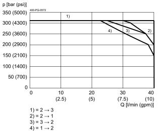
$\Delta p = f(Q)$  Pressure drop-flow rate characteristic ∆p [bar (psi)]
